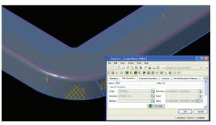
Fibersim provides automated methods for addressing manufacturing challenges. Darts, displayed as the two blue curves in the bend, are created while viewing material deformation.
