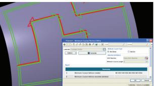
The Fibersim minimum course utility automatically identifies corners where material additions are required to ensure minimum courses can be laid up during automated fiber placement.
