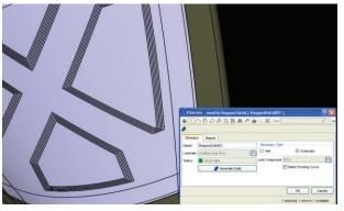
Fibersim provides a rapid method for assessing packaging and clash by automatically generating a stepped solid (gray) representation.
