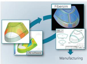
The Analysis Interface drives analysis from the same single CAD master model that is used for design and manufacturing. This permits analysis to be performed on a part in its to-be-manufactured state.
