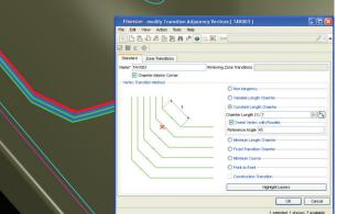
Modifying ply corners is as simple as selecting the desired chamfer or shape in Fibersim using its intuitive interface that immediately updates ply boundaries.
