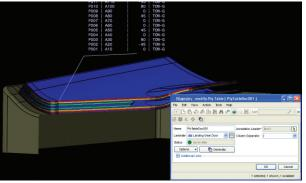
Fibersim exploded laminate and annotation capabilities provide an instantaneous method for creating surface representations of the stack-up and annotations that are updatable as the design changes. Plies are indicated by blue-0°, green-45°, yellow-90°, red-45°.
