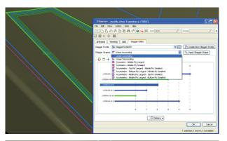
Fibersim zone transitions provide an automated way to create the desired drop-off profile by either using stagger shapes or dragging and dropping plies to the appropriate ply boundary.
