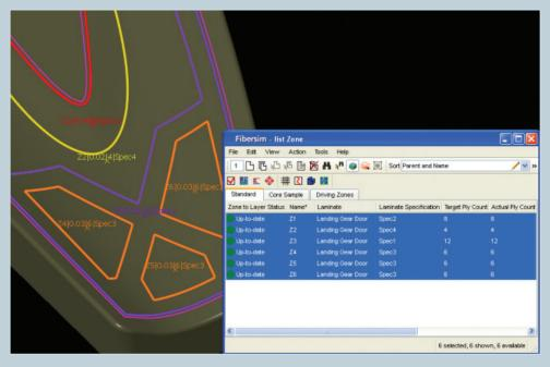
The Fibersim zone-based capability defines material specifications for specific areas of the part called zones. Zones highlighted in Fibersim are displayed within the CAD model in a user-defined color with text indicating the zone name, zone thickness, number of plies and specification.
