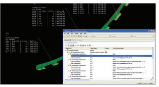
QPE automatically creates inspection characteristics – such as material type and ply orientation – for a shear tie of a composite fuselage based on ply information created in Fibersim or data extracted from specification tree formats or databases.
