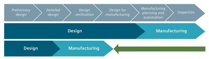
Fibersim compresses the design-to-manufacturing process for composite components by up to 45 percent.
