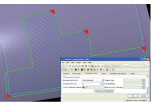
The Fibersim spine-based simulation is the only solution that allows you to identify areas of localized deformation (highlighted in yellow and red) that are caused by part curvature and fiber steering during manufacturing.
