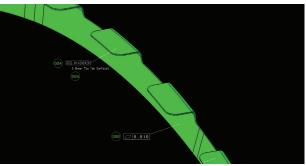
Dimensions, tolerances and notes defining design characteristics of the laminate are consumed into the QPE to provide a complete set of pre- and post-cure inspection requirements.
