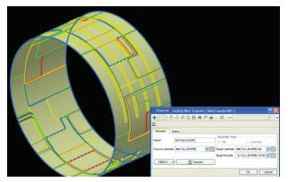
Fibersim parametric surface offset capabilities make it easy to create IML tooling (tan surface) and update it with design changes. The skin transfer capability automatically transfers the plies from the design definition (blue, yellow, green and red curves) to the manufacturing model.
