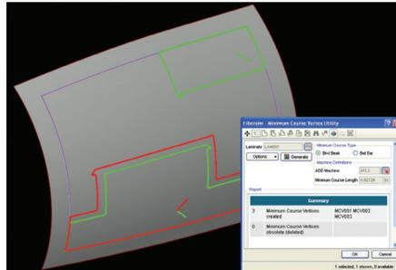
ADD has automatically identified where the machine will have minimum course limitations on this fuselage panel and has applied bird beaks to the corners of the  $\pm 45^\circ$  plies.
