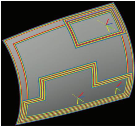
ADD has automatically added extended ramps to the outside edge of the plies on this fuselage panel to eliminate cliff edges and avoid material lift and smear.
