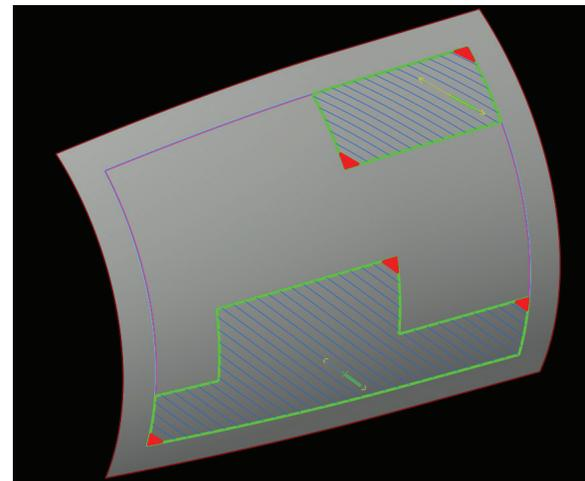
The course challenges simulation feature of the Composite Engineering Environment module in the Fibersim portfolio has identified in red the locations on this fuselage panel at which there will be manufacturing issues due to machine characteristics. The simulation provides the feedback needed to find and make the required changes early in the design cycle.
