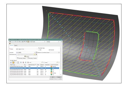
The Fibersim fiber placement import has brought the path planning centerline curves (blue), course edge curves (yellow), tow start points (green) and tow stop points (red) into the design environment for making additional design changes as required.
