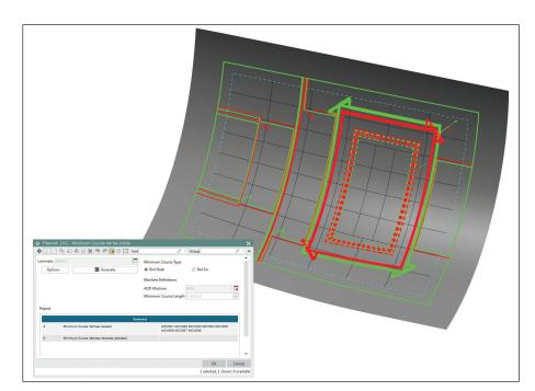
The Fibersim minimum course utility enables you to identify and change the corners of 45° layers (green) and -45° layers (red) layers that need their boundaries modified for manufacturing. The pinwheels or birdbeaks at the corners were automatically added.
