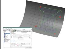
Manufacturing challenges with the design can be identified by using the characteristics in the Fibersim machine database. The areas of red in the corners of this 45° layer are highlighted, letting the engineer know that the design does not address short course limitations with the fiber placement machine.
