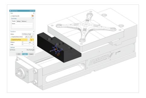
an additional edge that can be used to drive or define toolpaths. Likewise, trim, sew and join functions enable surface and edges to be modified to support NC operations.
