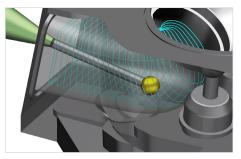
Tube machining streamlines programming of complex hollow regions typically found in manifolds, cylinder head ports and shrouded impellers.
