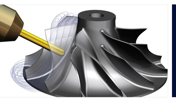
NX Turbomachinery Milling for easy programming of multi-bladed parts
