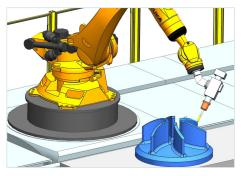
Program robots to machine large parts and to automate machining tasks typically performed manually, such as polishing, trimming and deburring.
