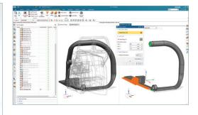
The lattice tool features several work-flow and command enhancements and enables users to place balls at the lattice nodes to further improve lattice durability. The tessellation factor is maintained between editing operations for improved lattice quality.
