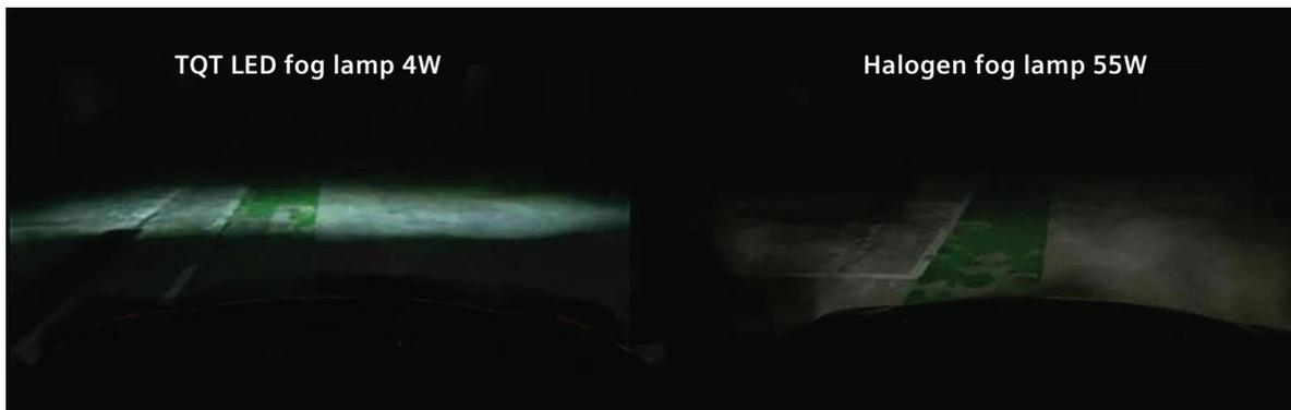
Figure 3. Car road-test comparison of the new TQ Technology LED fog light with a halogen fog light.
